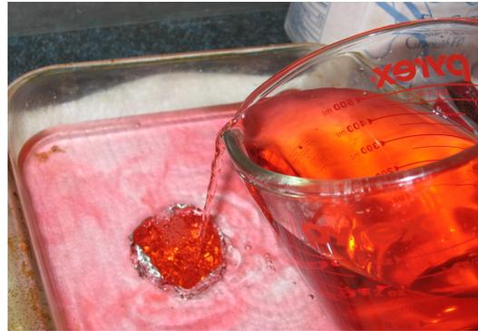
Figure 2: After filling the bottom half of the pan with sugar water, pour tap water, dyed red, into the aluminum boat. This will inhibit mixing and most of the red water will end up floating on top of the sugar water solution.
