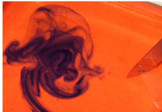
Figure 4: Dragging a knife through the patch makes more complex patterns of vortices.
