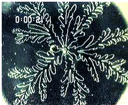
Figure 3: An experiment showing the nonlinear development of Saffman-Taylor instability in a non-Newtonian liquid. Courtesy of Peter Palfy-Muhoray and Roland Ennis (Liquid Crystal Institute, Kent State University).
