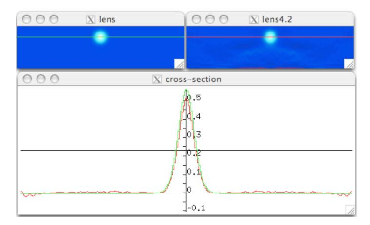
$c(x_1, x_2) = c_0 - a \exp(-(x_1^2 + (x_2 - 0.5)^2)/0.09), a = 0.4, c_0 = 2km/sec$
