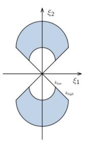
If the source wavelet q has frequencies down to 0, f can be recovered from 2 plane waves making an angle of 90°.
