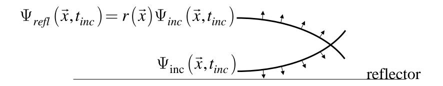
$$\frac{\Psi_{refl}\left(\vec{x}, t_{inc}\right)}{\Psi_{inc}\left(\vec{x}, t_{inc}\right)} = r\left(\vec{x}\right) \quad \text{A reflectivity estimate.}$$
