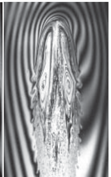
Figure 6: A nylon fiber being deformed by the oncoming flow of a running soap-film.
