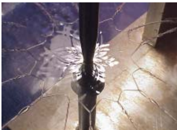
Figure 1: Fluid hits a flat plate, and is expelled sideways. From “Fluid polygons”, by R. Buckingham and J. Bush, Physics of Fluids 13, S10 (2001).
