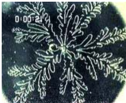
Figure 3: An experiment showing the nonlinear development of Saffman-Taylor instability in a non-Newtonian liquid. Courtesy of Peter Palffy-Muhoray and Roland Ennis (Liquid Crystal Institute, Kent State University).
